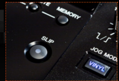
Slip mode allows scratching without affecting track length or losing the beat
